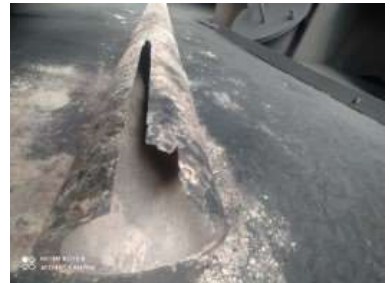
(iii) Failure of Stainless steel pipe/nozzle
